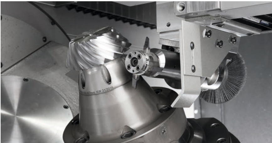
Fig. 4: Flexible deburring in the machine
