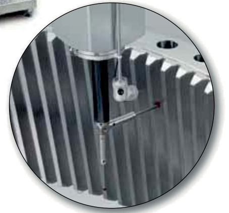
Fig. 4: Measuring arm with monitoring camera
